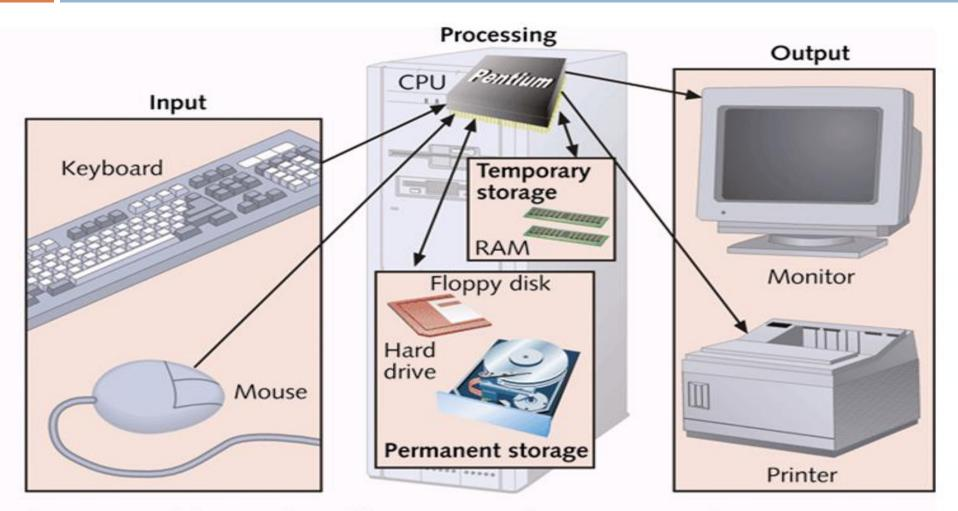
Computer activity consists of input, processing, storage, and output
